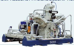
Large/medium size mechanical compressors equipped with 2 or 3 cylinders positioned at 60°. SWSE series compressors compared to SW are equipped with single-effect cylinders that allow easier maintenance, reducing operating costs. These compressors are suitable to operate with low suction pressures.
